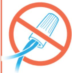
**IMPORTANT:** If your thermostat is built into the wall and connected to thick wires with wire nuts, or if it is labeled 110, 120, or 240 volts, you have a high voltage system that is **not compatible** with the GLAS Thermostat. Do not connect your thermostat to these high voltage wires. GLAS is only compatible with 24VAC systems.
